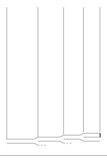
The forward compression wavefront begins at the root of the tree with magnitude 1. Because the bifurcations are well-matched, it travels without change through all of the vessels of the tree.
