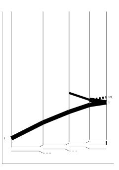
The backward compression wavefront in the  $3^{rd}$  generation vessel is reflected when it arrives at the  $2^{nd}$  bifurcation with R = -1/2, producing a forward decompression wave of magnitude 1/4. This wave propagates forward without change until it encounters the occlusion.
