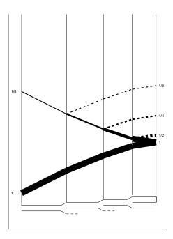
The reflected forward decompression wavefront of magnitude 1/4 that arrived at the occlusion will generate a sequence of wavefronts exactly like the original wavefront of magnitude 1, except that the magnitude of each wavefront will be reduced by 1/2 and the sign of the wavefronts will be inverted. I.e. compression wavefronts and decompression wavefronts will be compression wavefronts.
