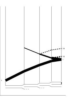
The backward compression wavefront with magnitude 1/4 is similarly reflected and transmitted when it reaches the  $1^{st}$  bifurcation. The reflected wavefront is a decompression wave of magnitude 1/8 and it propagates forward without change until it reaches the occlusion. The transmitted wave propagates backward to the root of the tree. The first result of the occlusion at the root of the tree is therefore the arrival of a compression wavefront of magnitude 1/8.
