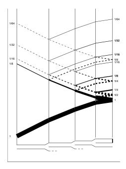
The twice reflected wavefront arriving at the occlusion as a compression wavefront with magnitude 1/4 will also generate a similar family of wavefronts to that produced by the original wavefront but with magnitudes reduced by 1/4. This will produce a compression wavefront arriving at the root in between the first two decompression wavefronts already described. It will have magnitude 1/32.
