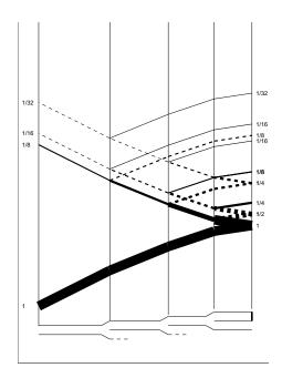
The reflection of the first reflected wavefront from the  $1^{st}$  bifurcation, a decompression wavefront of magnitude 1/8, will generate another family of wavefronts with magnitudes reduced by 1/8. This will generate a decompression wavefront arriving at the root with magnitude 1/64.
