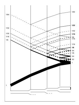
The next compression wavefront to arrive at the root of the tree is generated by the re-reflection of the backward decompression wave from the  $2^{nd}$  bifurcation. It will have magnitude 1/64.
