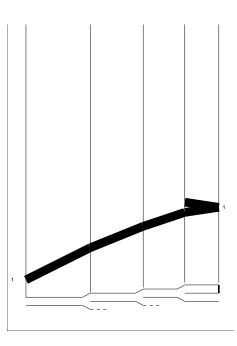
At the  $3^{rd}$  bifurcation the reflection coefficient is R = -1/2, so the backward compression wavefront generates a reflected decompression wavefront of magnitude 1/2. The transmission coefficient is T = 1 + R = 1/2, so a backward compression wavefront of magnitude 1/2 is generated in the  $3^{rd}$  generation vessel.
